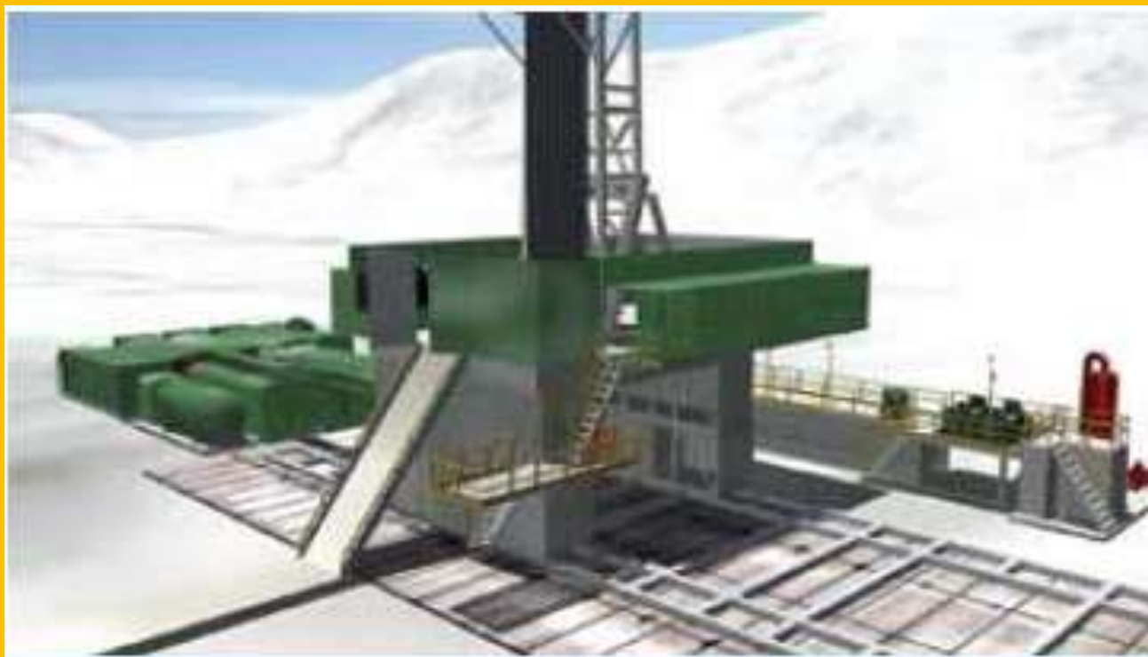
Fig. 1. The PaDSRig (Production and Drilling System Rig) is designed for drilling multiple well bores from a single pad location, skidding along rails.
